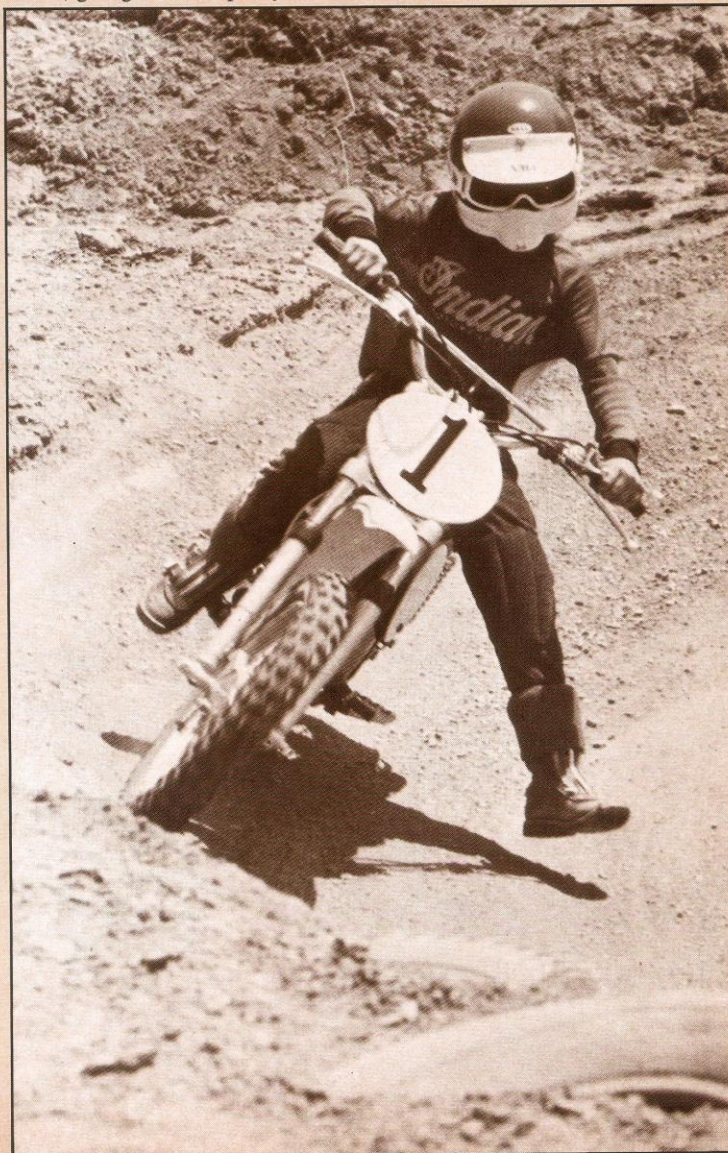
Forged alloy triple clamp and crown securely grip the fork legs, helping to prevent any front end wobble.
