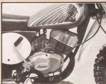
The 49.6cc two-stroke engine is a tight fit in the double-loop frame. A four-speed close ratio gearbox is standard.
