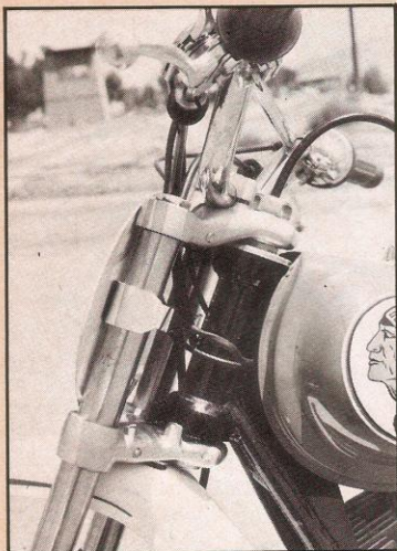
Forged alloy triple clamp and crown securely grip the fork legs, helping to prevent any front end wobble.
