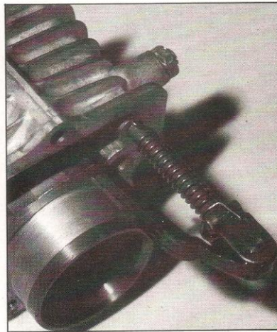
14) View of cylinder showing timing chain tensioner. The bolt coming out of the back of the cylinder is a second adjustment for tensioning the timing chain.
