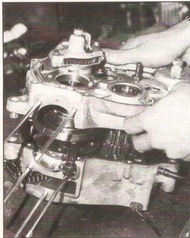
22) After breaking the seal, gently lift off the engine case half, making sure you do not disturb the transmission shafts.
