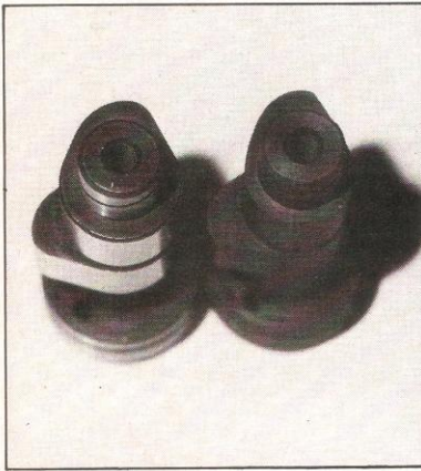
1) On the right is the re-ground Hacienda cam, treated with black slippery stuff. Compared to the stock cam (left) some idea of the increased valve lift and quick closing can be obtained.
