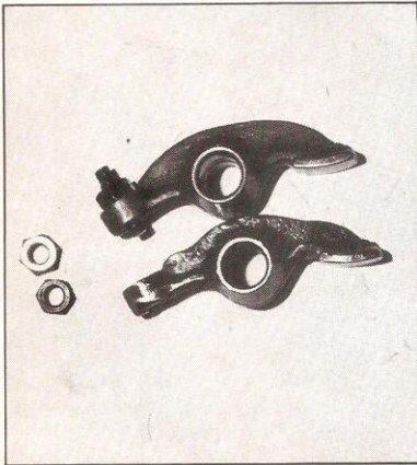
4) Top is the stock rocker arm, below the lightened version. The differences are subtle but important. In the search for light weight, the smaller adjusting nut on the bottom is used.
