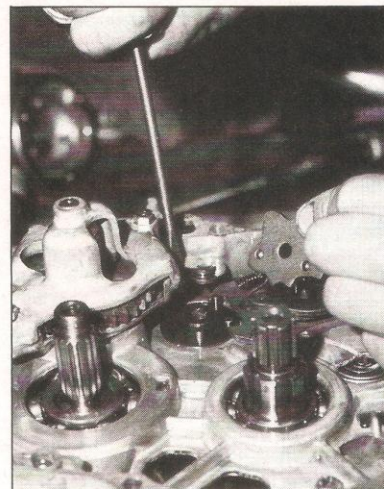
26) Holding open the ratchet roller arm with a screw driver, the ratchet plate is installed so that the two locating pins fit into the plate.
