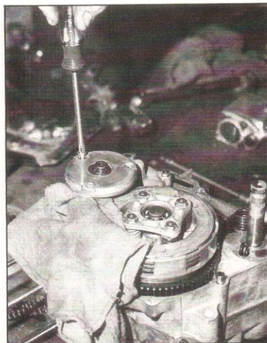
17) With a rag jammed between the primary gears to prevent things from moving around, remove the oil pump filter cover.
