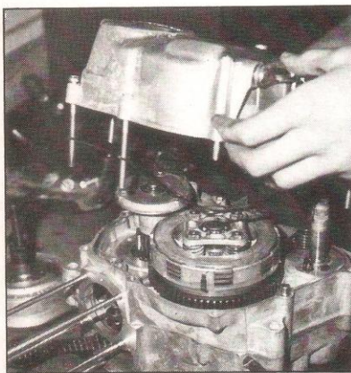
16) After removing the flywheel with a puller available from Honda dealers (seen laying on the bench to the left), unscrew the clutch housing. Note that the long clutch housing screws also serve to hold the engine case halves together, with only two retaining screws located under the clutch housing.
