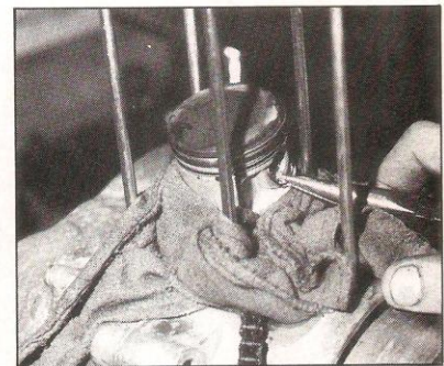
15) If "Platinum Blonde" modifications are to be carried out, there is no need to maintain tension on the timing chain since the crankshaft will be removed. Here the piston is being removed. Although the engine case will be split, it is a good idea to prevent carbon and dirt from entering the lower end by stuffing the top of the case with rags. The piston wrist pin locking clip is removed by a twisting motion on needle-nosed pliers.
