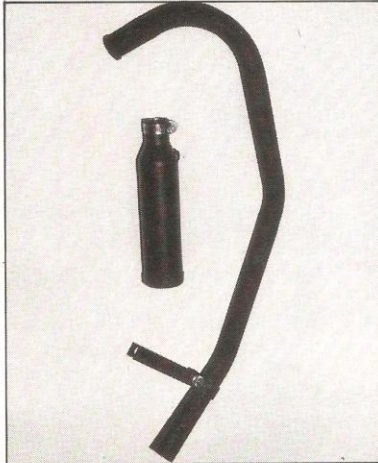
2) Hacienda exhaust system. The pipe is straight through and the appearance of flare at the end is due to shadow.
