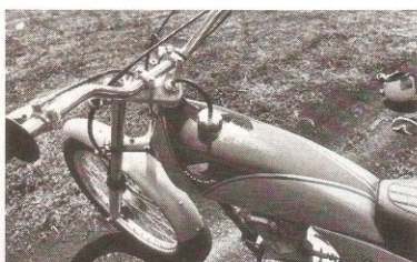
About the best front end found on lightweight trials machines. Note lean gas tank.
