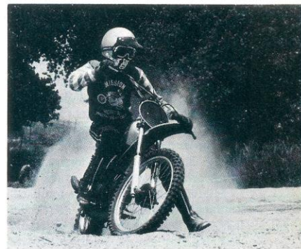
The tall gearing is good for quick starts in soft sand because it minimizes wheelspin.
