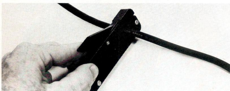
Hook-up to the engine is simple. Place the black box over the spark lead and be sure that the jaws are closed.
