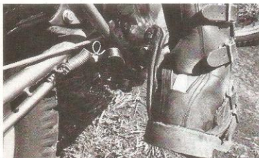
Looks like an afterthought but the little spring did a neat job of holding the footpeg up while the kickstarter gets a good swing.
