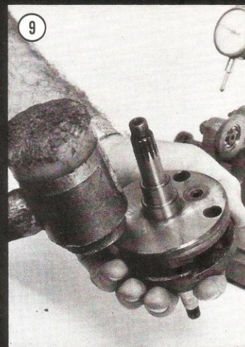
Tap the flywheel on the side at the point where run-out is greatest.
