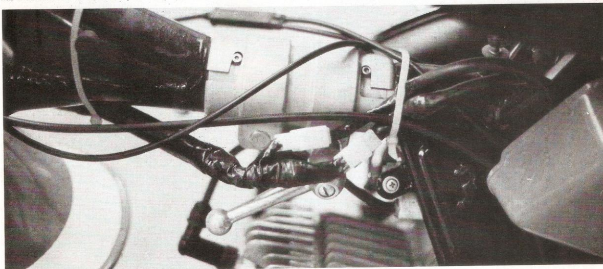
The heart of every conversion is this simple, quick-disconnect yoke for the frame. Assembly takes as little as five minutes for the experienced.
