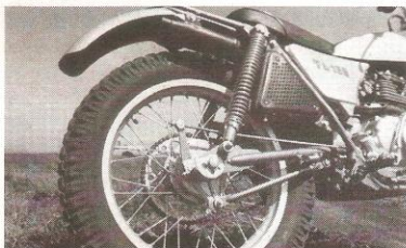
Rear shocks were only average. Machine need more forgiving rear suspension. Note tucked-in muffler.
