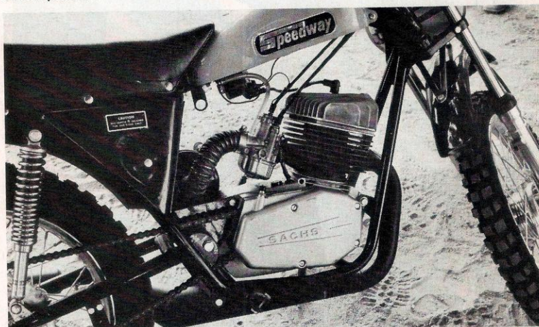
The 125 Sachs engine with 5-speed has been around for years in the winning bikes.
