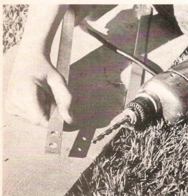
M. Braces for trailer hitch are drilled to mount on the upper shock absorber bolt.
