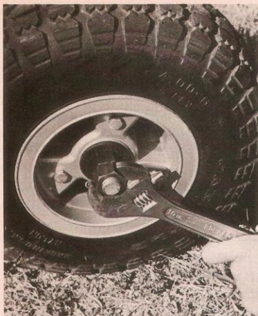
F. Wheel is double-nutted to lock it into place on the end of the axle.
