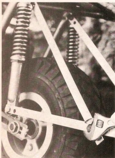
Q. Brace runs from upper shock mount to back of trailer hitch.
