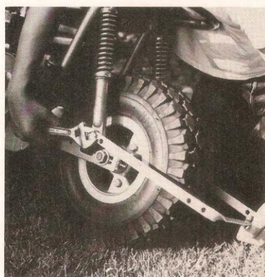
P. Hitch is mounted on lower shock absorber bolts - trail machines will have suspension.
