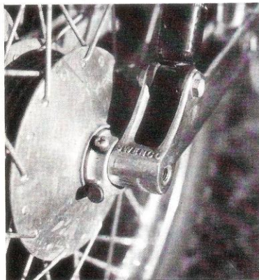
BELOW - Deep axle bearing with the speedo sender unit still in place.
