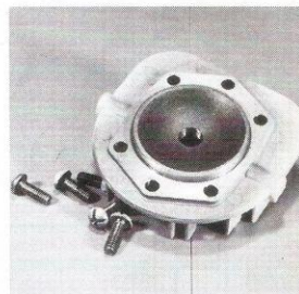
LEFT - Although there appears to be an eight screw head hold-down pattern, only six screws are actually used. This is discussed in the text.
