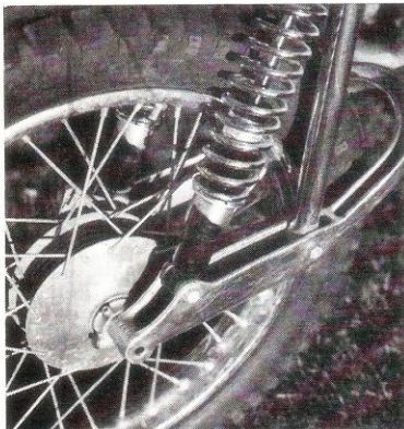
ABOVE - The sturdy construction of the channelled (for weight reduction) die cast swinging arm can be seen here.
