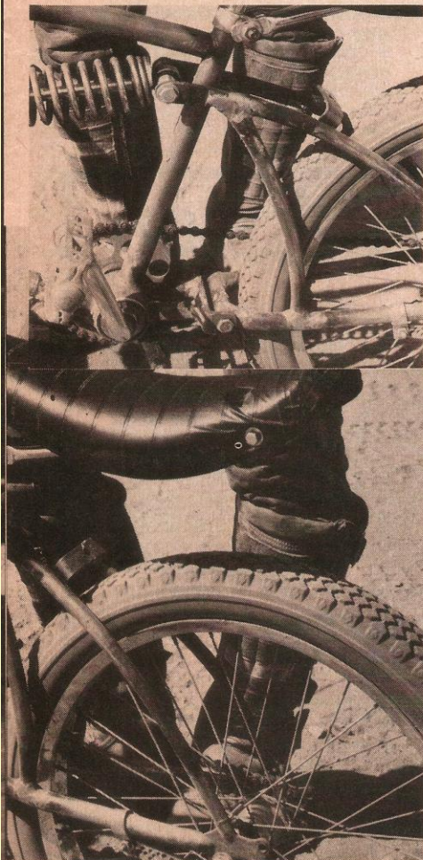
At this stage the frame welding looks a little crude because it hasn't been painted and filed clean, but the system works beautifully.
