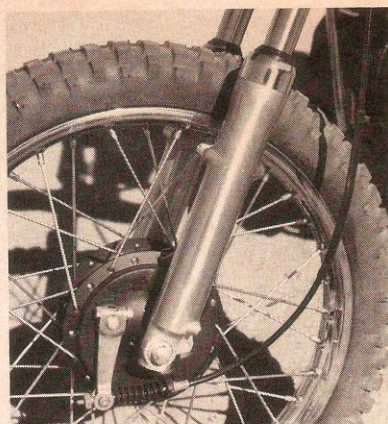
Front shocks are oil-dampened but "squishy." Note brake wear limit marking.
