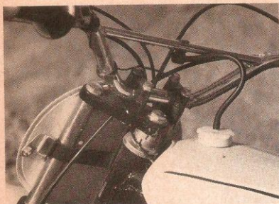
Giant rubber band holds number plate simply and securely.
