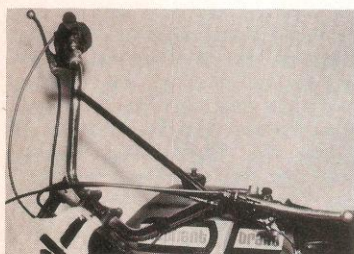
CONTROLS - Mounted on the motocross handlebars are standard Hodaka controls, replacing the Bonanza units.
