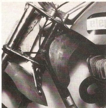
GUSSETTING - Half-moon gussetts behind the steering head and additional welding at the steering head, prevented fractures.
