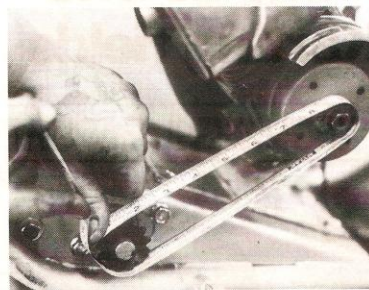
CHAIN - Length of chain being measured. Alignment of sprockets is critical.
