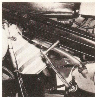
POLLUTION CONTROL - Plastic tube over dip-stick location prevents cold oil from seeping. Note mudguard over rear fender.
