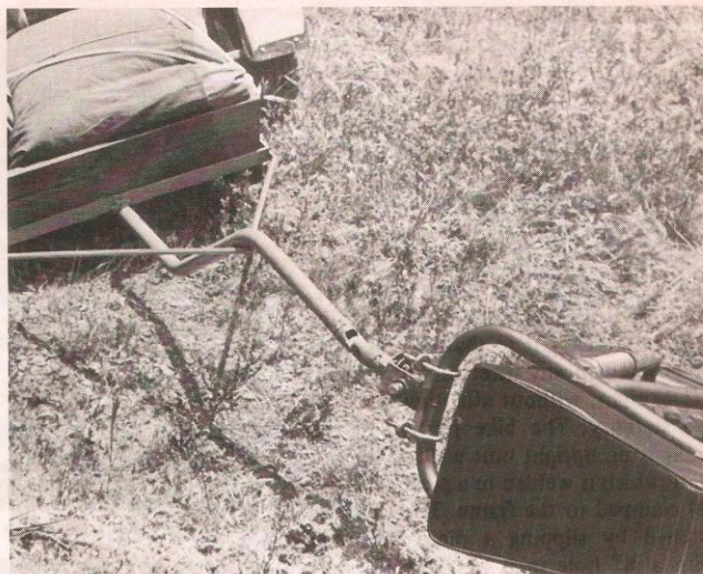
FREE - Use of universal joint and pivoting end bolt allows the mini-bike freedom.
