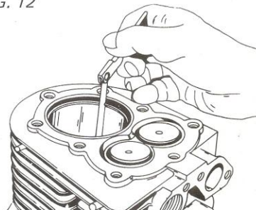
GAUGING END GAP ON RINGS
