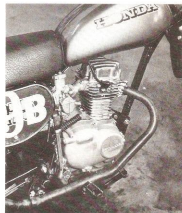
The bike we chose to do the work on already has a megaphone exhaust but otherwise the engine is stock. Start the work by removing the exhaust pipe and megaphone. Two bolts hold the flange in place and one bolt holds the pipe to the frame.
