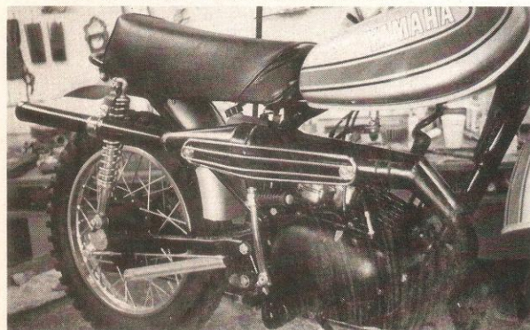
21) Huge Turner pipe is bulky but effective. Heat shields offer some protection to the rider's leg. The long stinger-silencer helps tame roar.
