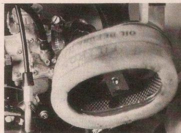
4) Greatly increased volume of air box and giant filter are a necessary part of the modified intake system.
