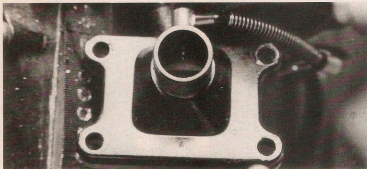
7) This peep-hole is where the standard carb mounts to the reed cage.
