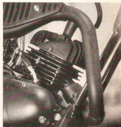
18) YZ's standard exhaust system features a very long head pipe which provides a flat power curve.
