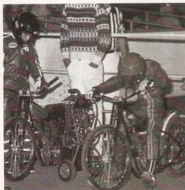
Battery starter kicks over McCulloch engines of these 3/4 scale racers.
